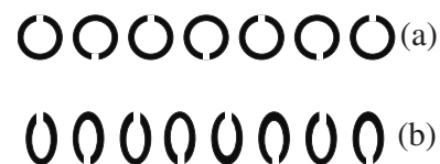
FIG. 1. Schematic of a one-dimensional array of split-ring resonators in (a) planar and (b) axial geometries. The axes of the split-ring resonators as well as the magnetic component of the applied field are directed in parallel. The electric field component is transversal to the slits.
